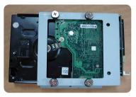
2. When assemble the SATA converter board, screw on the only upper-right corner like the picture below.
